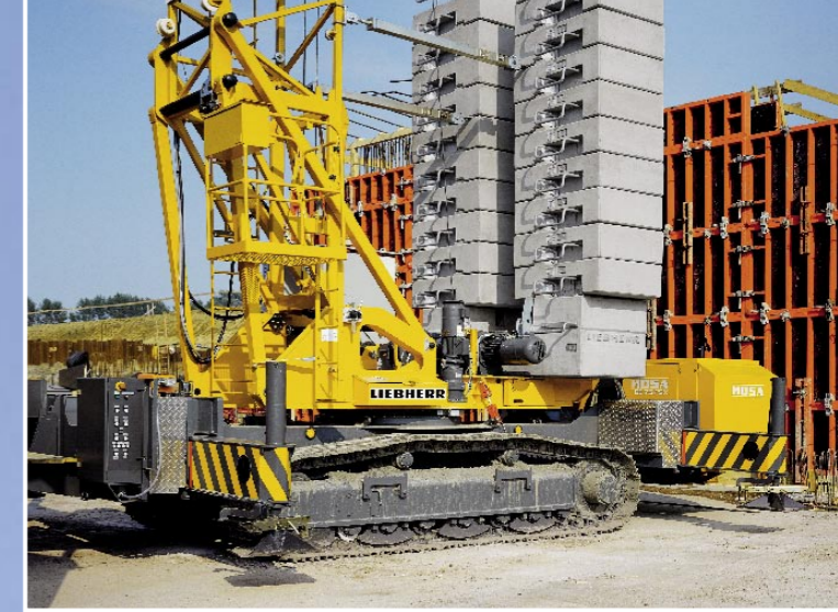
The 42 KR.1's compact crawler travel gear.
